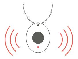
Turn the MobileHelp PERS unit over to slide the power switch to **ON**. Wait for the unit to announce "System Ready" to proceed.
